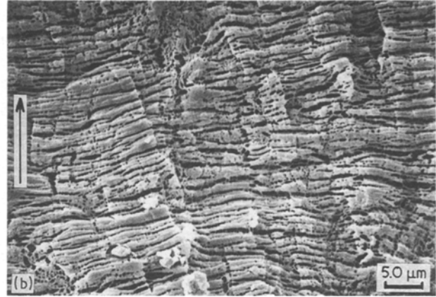
Figure 6 Typical fatigue fracture surface topography of POM (arrows indicate growth direction) (a) regions I and II of crack growth, (b) region III of crack growth, (c) region of catastrophic failure.
